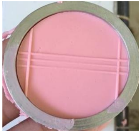
Figure 1. The alginate mold's surface was observed to determine its adherence to the ADA specification 50 m line (Doc)
